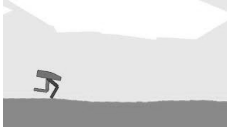
Figure 19: OpenAI virtual Bipedal Walker environment. An environment where motor control is inputted into the environment to cause the walker to move steps.
